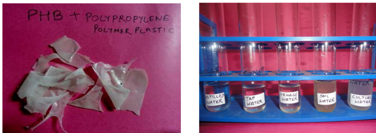
Fig 7. A) A film of blended mixture polyhydroxybutyrate and poly-propylene polymer plastic, B) Biodegradability Analysis of of Agri-bioplasic.
